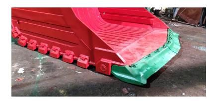
Key features of an LHD excavator bucket include its design for optimal scooping and loading of materials, often with a higher capacity than standard buckets. The bucket is part of the LHD machine's system, which typically includes a front bucket for loading, a hauling mechanism, and a dumping system. LHDs are well-suited for confined spaces in underground mining environments, where efficient and precise material handling is crucial.
